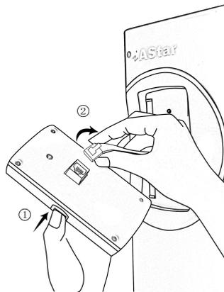
Fig. 3-6 Disconnect operator
