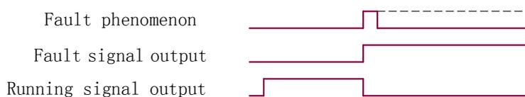
Figure 7-15 Time sequence of fault signal
