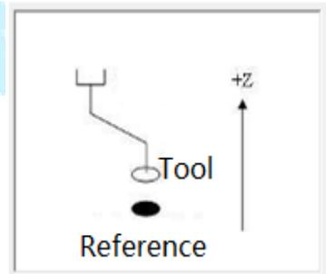
3. Under Right-hand frame, adjust the tool tip again coinciding with the reference point, click on the "P2" (location assigned to the P2). Calculates the tool parameters (X/Y/Z/C) records in the selected row.
