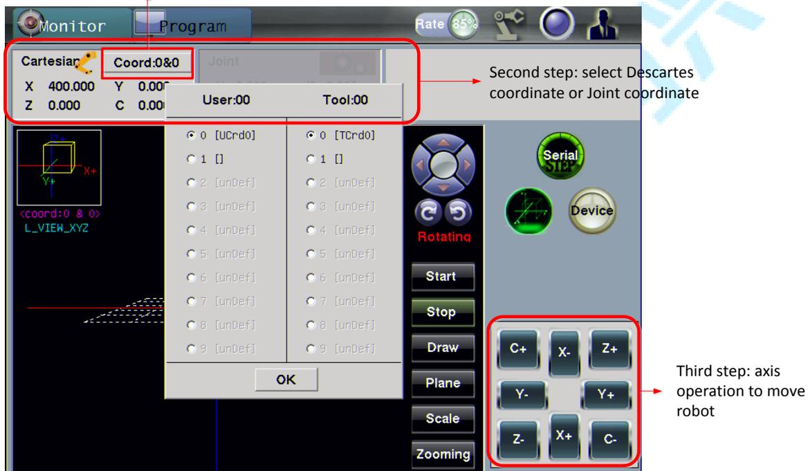
For Descartes/joints manually, it involves some other operations, such as continuous/step switching, rate changes, and so on.
