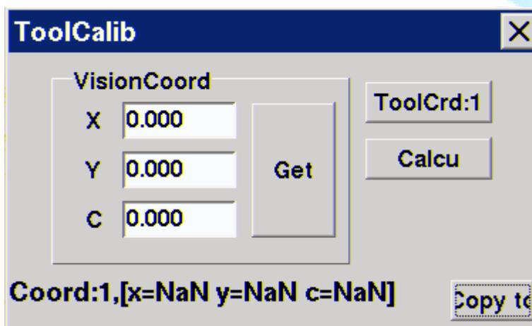
**Note:** function of “Copy to” is used for saving the calibrated tool result to DATA.PTS.
