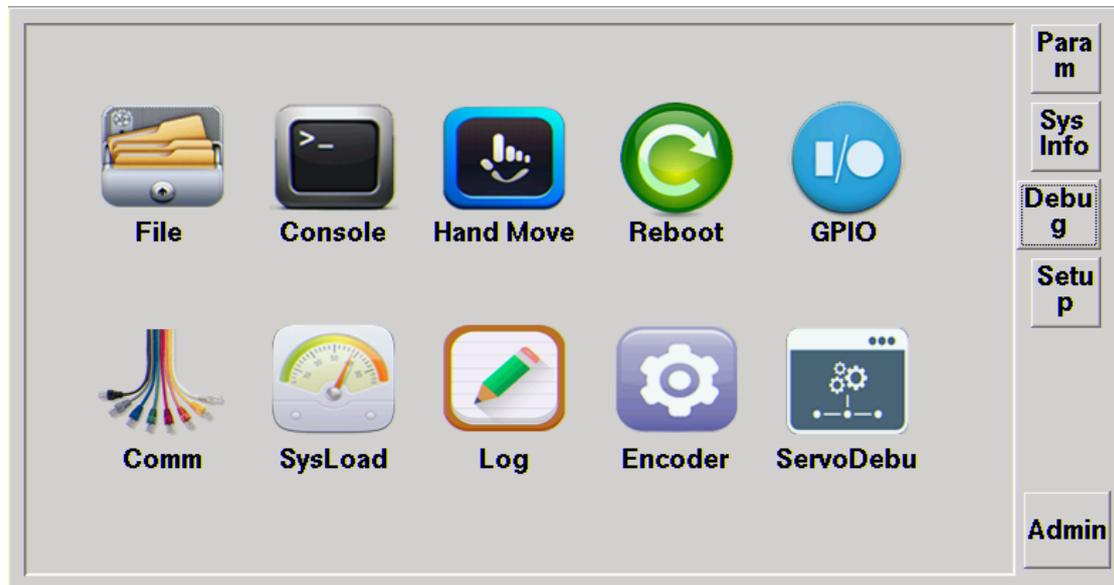
Debugging tools are some auxiliary tools in the robot debugging process, including file management tool(**file**), system debugging information(**Console**), manual debugging (**HandMove**), GPIO, communication station(**Comm**), encoder information(**Encoder**) and Servo debugging(**ServoDebug**).
