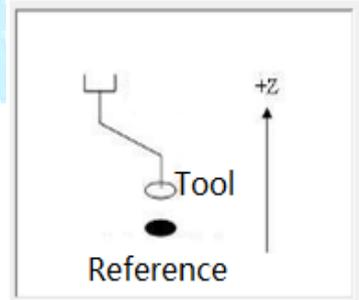
3. Under Right-hand frame, adjust the tool tip again coinciding with the reference point, click on the "P2" (location assigned to the P2). Calculates the tool parameters (X/Y/Z/C) records in the selected row.
