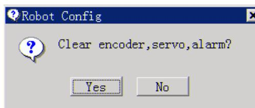
Press “Yes” to clear encoder, servo, alarm. This case is applied for roughly calibrating the home position of the robot once home has lost.
