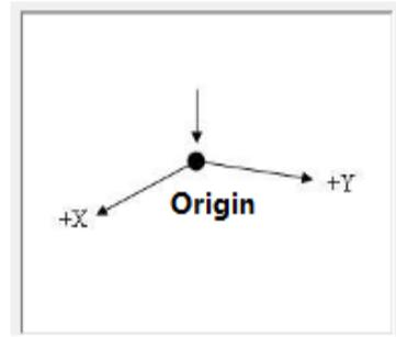
4) Select “xx” in “UserCalib” interface; Then move along the x-direction of the workpiece to reach a appropriate position; Then click on “Teach” to assign the current robot’s position to “xx”. Notice that C-axis is forbidden to be rotated, or it will lead errors during calculation.
