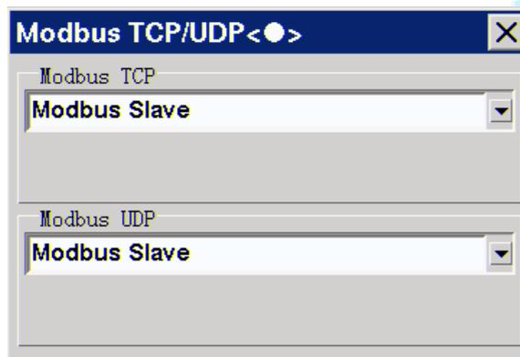
(2) When robot is Poll station, the corresponding parameters should be set as follows:
