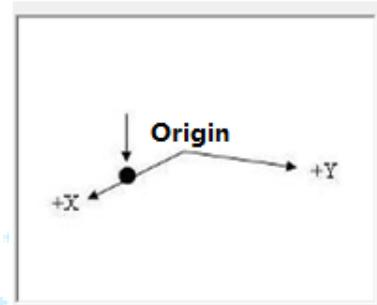
5) Select “yy” in “UserCalib” interface; Then move along the x-direction of the workpiece to reach a appropriate position; Then click on “Teach” to assign the current robot’s position to “yy”. Notice that C-axis is forbidden to be rotated, or it will lead errors during calculation.
