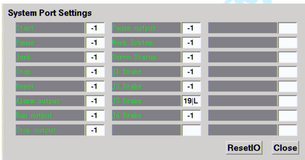
Click “ResetIO” to enter ResetIO interface. In this interface, you can open(ON) or close(OFF) all outputs.
