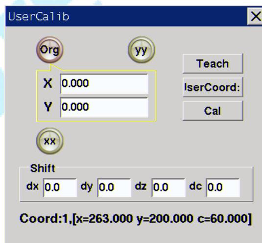
Tips: if a camera can return the coordinates which is referred to base coordinate of robot, the calibration of user coordinate can be ignored.
